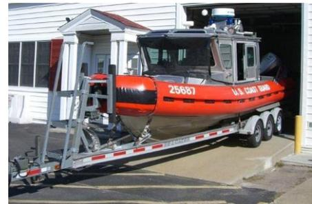
**8. Keep the boat motor off the pavement.** Some motors can be left in the vertical position in transit, but many large motors need to be tilted up so that the skeg doesn't drag on the highway. If you need to tilt up the motor, avoid too much stress on the transom with a support bar that fits on the last roller of the trailer. A motor support bar puts the load on the trailer and relieves any stress on the transom.
