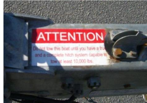
**3. Opt for a strong hitch.** The Motor Vehicle Manual, COMDTINST M11240.9C, Appendix C, provides a Trailer-Truck-Hitch Matching Checklist. Hitches are rated as Class I, II, III, IV, and V. Class V has the greatest towing capacity and is required for SAFE boat trailering. Two suggestions to prevent mismatched hitch and ball are to standardize the hitch/ball combination to one size or to color code the hitch and ball.
